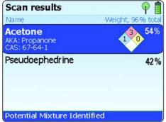
TruDefender FT provides clear results which require no user intervention. Each analysis automatically checks for the presence of mixed chemicals.
